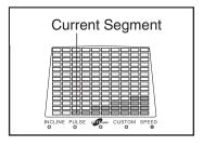
incline settings will not be shown in the matrix.) The speed settings for the next seven segments will be shown in the columns to the right. **If an incline program is selected**, the incline setting for the first segment will be shown in the flashing Current Segment column of the matrix. (The speed settings will not be shown in the matrix.) The incline settings for the next seven segments will be shown in the columns to the right.
